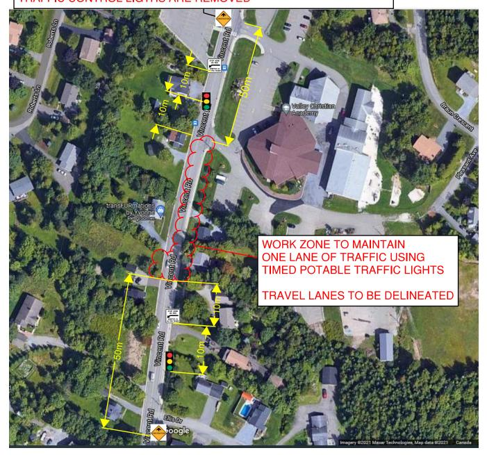
TRAFFIC DISRUPTION TO LAST APPROXIMATELY ONE WEEK DURING THE INSTALLATION OF SAMH-3 AND 250MM DR21 FORCE MAIN PIPE. FUTURE DISRUPTION FOR MILLING, GRADING AND PAVING TO LAST NO MORE THAN ONE WEEK
